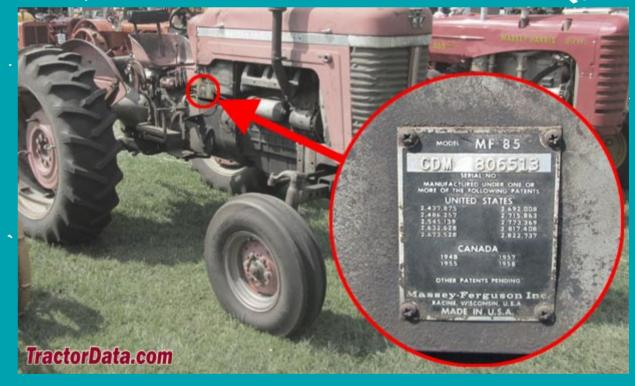
On the upper right is a photo of a Massey Ferguson that can help you identify where the information will be. With the serial number, you will need to find the dealership model chart to find out the specific year and model.
